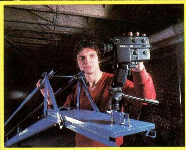
Ken Walker with his completed "Walkerflex" camera crane. Note the tripod head that Ken mounted to the camera end of his crane for added versatility of movement. The crane can be built for about $75 with easily found materials.
