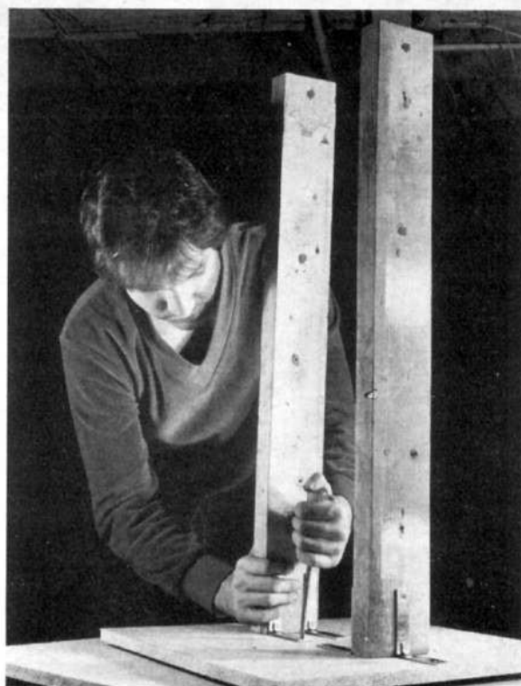
Walker screws the support posts to the baseplate of the camera crane, using strong steel "L" brackets for sturdy construction.
